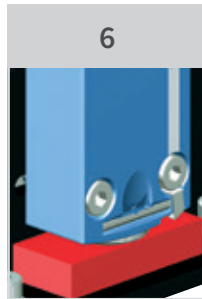
6 Enclosed fitting, resistant to dirt penetration
