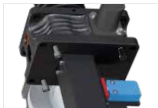
Blind tapped holes (ZE- and GSZ-Series): Z and GSZ series can be attached from underneath using the blind tapped holes in the gearbox. ZE size 5 to 25, GSZ-Series: all sizes
