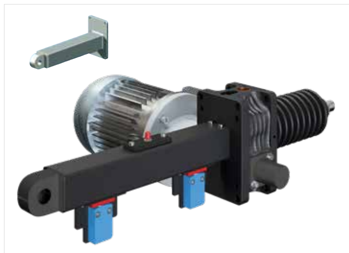
The pivoting support tube STRO has the advantage that the pivot points are entirely external. The disadvantage is that the gearbox and motor weights are in the centre. The manufacture is always customer-specific.
