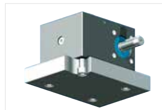
Blind tapped holes (ZE- and GSZ-Series): Z and GSZ series can be attached from underneath using the blind tapped holes in the gearbox. ZE size 5 to 25, GSZ-Series: all sizes
