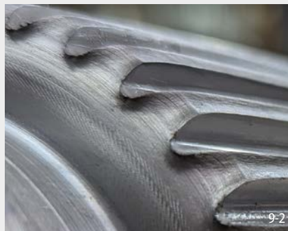
Detail view of a cold-rolled splined shafts
