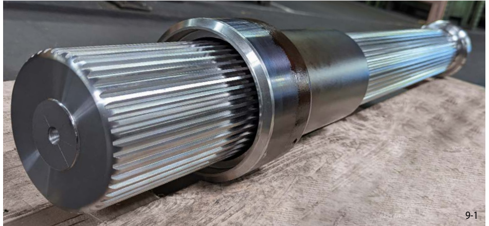
Hobbed splined shaft with splined sleeve in extra-long design.
