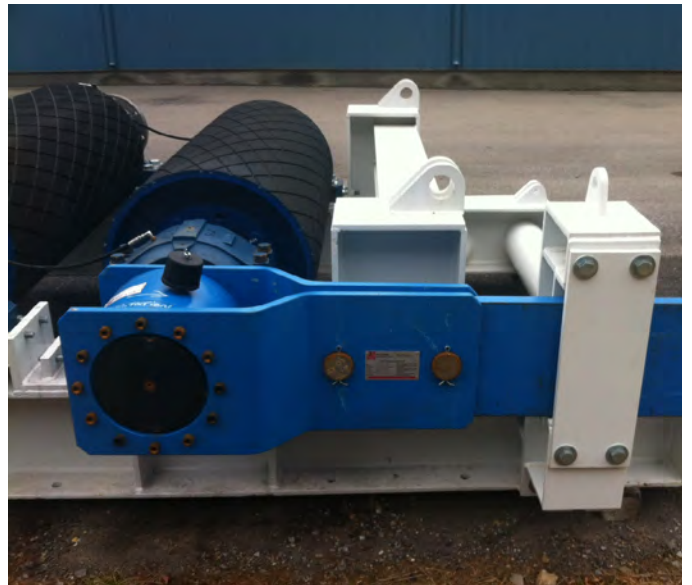
Low Speed Backstop FRHD 1000 in Incline Conveyor
