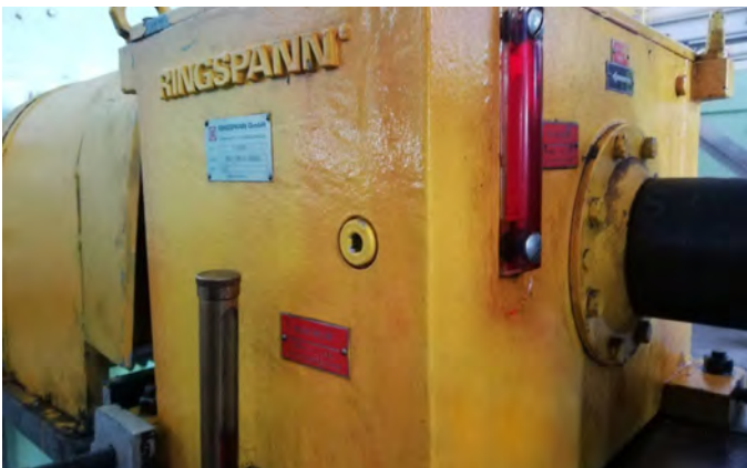
Housing Freewheel FH 4000 in hydraulic turbine pump
