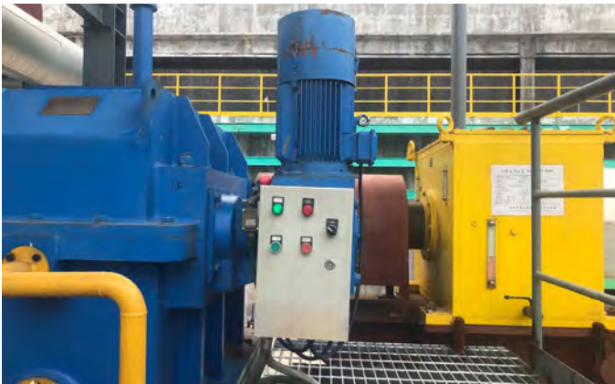
Housing Freewheel FH 8000 in water pump
