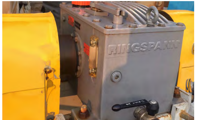
Housing Freewheel FH 1000 in hydraulic turbine pump
